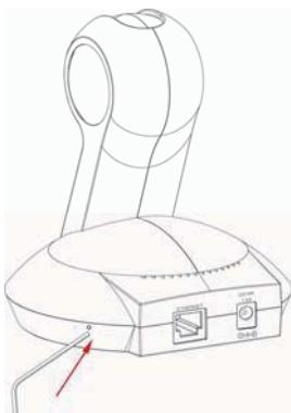
There is a button in the back side of the Network Camera. It is used to reset the system or restore the factory default settings.
