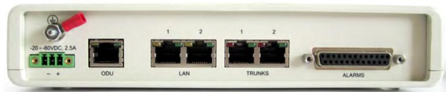
**Figure 3-11: New style IDU-E: Rear panel**
