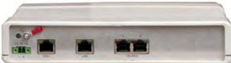
**Figure H-2: Typical IDU-E Rear Panel**
