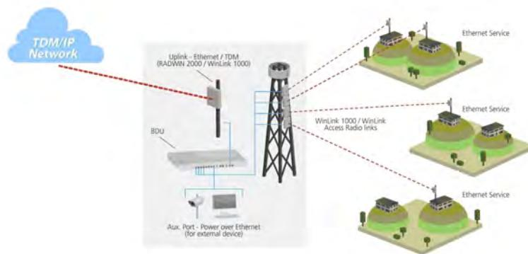
**Figure 1-20: Typical Multiple Point-to-Point deployment with wireless uplink**
