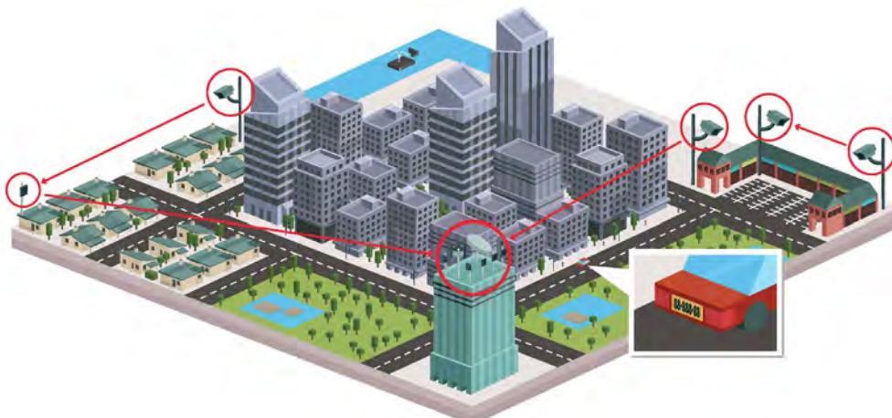
**Figure 1-4: Multi Point-to-Point Video Surveillance Deployment**
