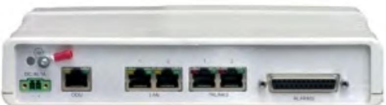
**Figure H-3: IDU-E-AL with Alarms port**
