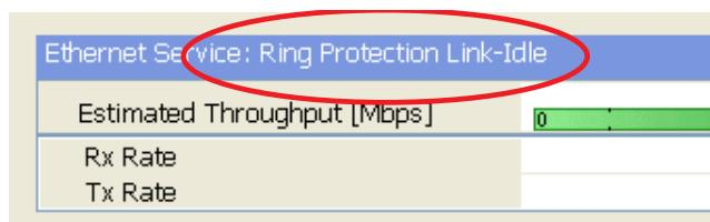
When the RPL cuts in as a result of a failure, the "Ethernet (Blocked)" notice disappears. The Ethernet Services Bar indicated that the RPL is active:
