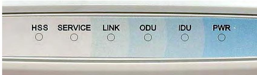
**Figure 3-15: IDU-E Front Panel LEDs**
