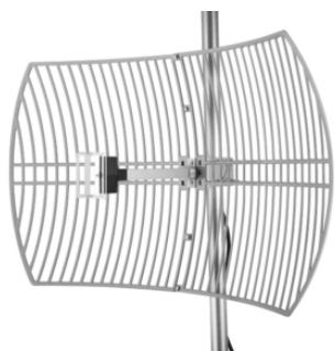
Grid antennas are used for 2.4 GHz applications. Due to the large size, the grid design minimizes weight and wind loading.
