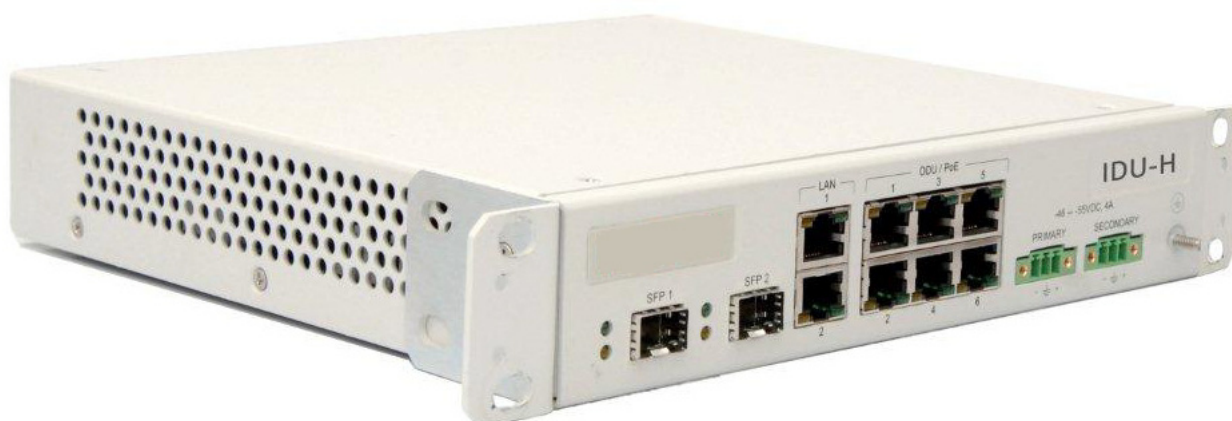
Figure 3-10: IDU-H front view - single configuration
