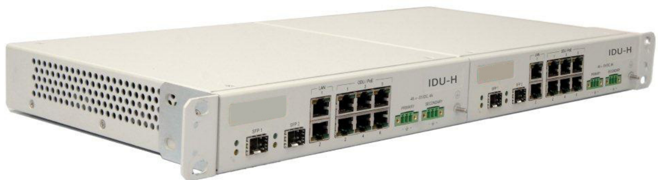
Figure 1-7: IDU-H front view - double configuration
