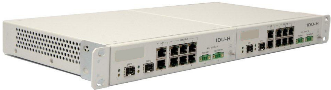
Figure 3-11: IDU-H front view - double configuration
