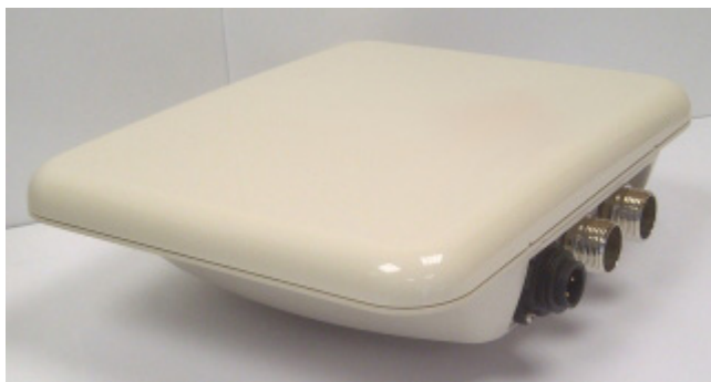
Figure 1-5: Small form factor HSU with AC power feeding
